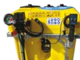
Motorized valves "Compact" for opening/closing right and left – for tractors with cabins.
