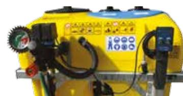
Motorized valves "Compact" for opening/closing right and left - for tractors with cabins.
