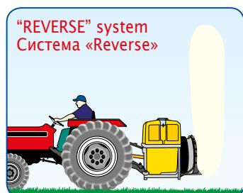
Nozzles don't spray against the tank like the traditional mist blower sprayers. With the system "Reverse" the chemical mixing is not directed to the tractor. Moreover this system avoids the problem of leaves, residual grass and dust from sucking up from the ground.
