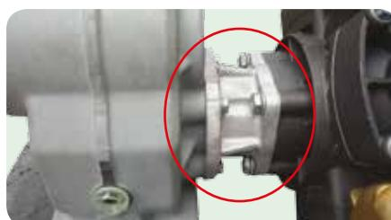
Direct connection between pump and gearbox for a strong support.
